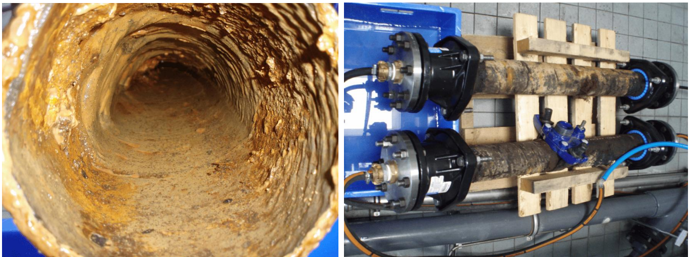
Figure 1. (a) DN 100 steel pipe upon delivery, (b) sequential arrangement of 2 * 1 m DN 100 steel pipes.
