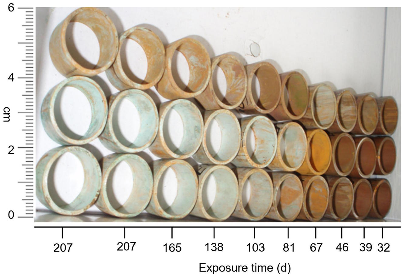
Figure 2. Corroded copper segments after exposure in Water 1, 2 and 3 (from bottom to top).
