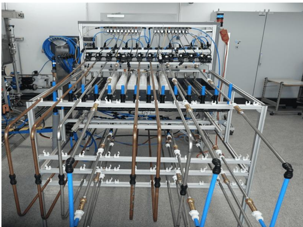
Figure 6. Corrosion test rig in accordance with EN 15664-1 from TZW, Karlsruhe.
