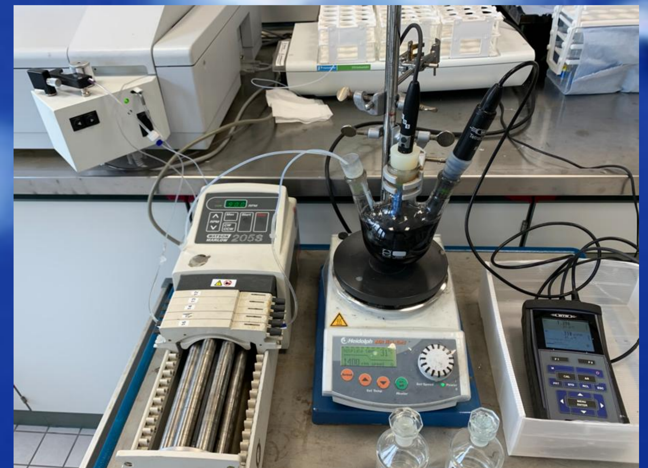
Picture 1. Experimental setup for measuring the kinetics of GNP with metalates.
